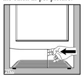
To pull out the condenser, first turn the two red stops inwards as shown below and then remove the condenser unit holding it at the handle.
